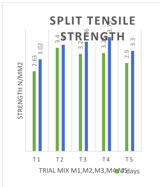
Graph 3.2 : Split Tensile Strength of Concrete at 7 and 28 day
