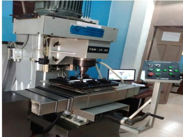
Fig.1. Friction stir welding machine setup
