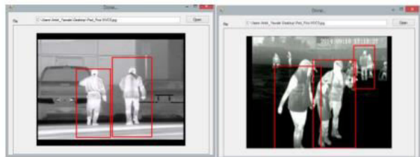
Figure 12. Processed frame of IR Night vision Camera and People are detected and labelled by Red rectangle
