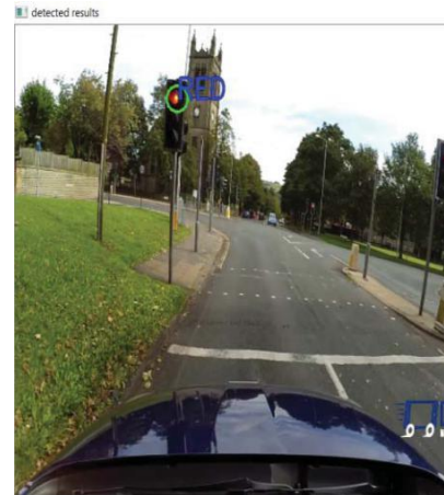
FIGURE 1: The Red Color Traffic Signal is Detected.
