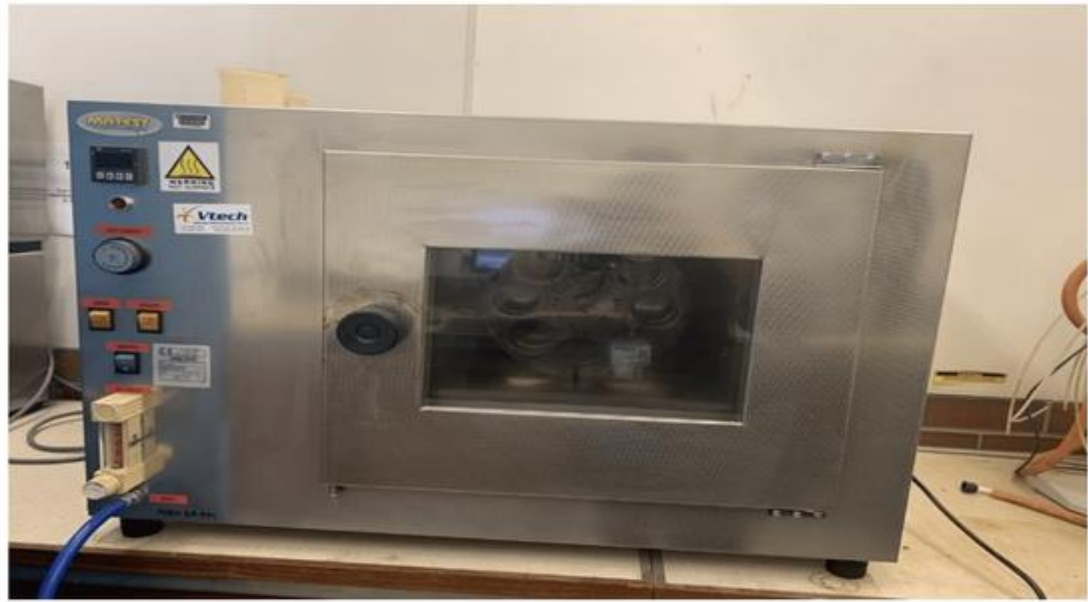
Figure 1-Apparatus of the RTFOT test
