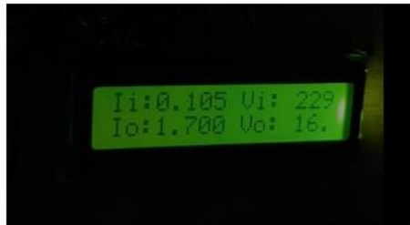
Notification through buzzer at set threshold (1.70 Amp)
