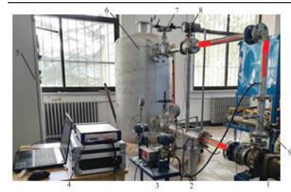
Figure 6. Test bench. 1. Model pump, 2. Pressure sensor, 3. Torque power meter, 4. Noise data sampling analyzer, 5. Power cabinet, 6. Water storage tank, 7. Flow control valve, 8. Electromagnetic flow meter, and 9. Hydrophone.
