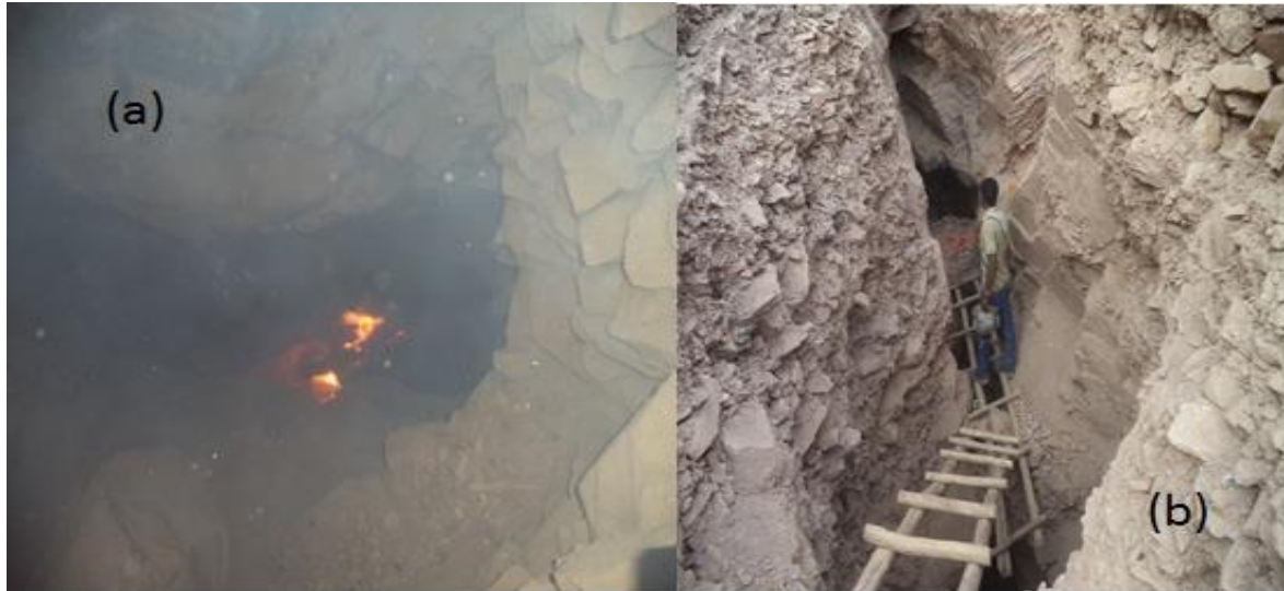
Figure 4: (a). Light oil used for firing the host rock, (b) deep shafts with competent host rock (Photo) Miner also sustained injuries from falling rocks and sharp tools, and have fallen into shafts. They worked with very unstable and troublesome formation within depths about 35 meters shown in Figure 5. Consequently, they risk grave injury when working in unstable shafts, which sometimes collapse or prone to slope failure.
