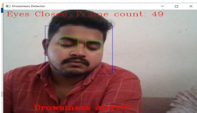
Figure 3: Test score increases above threshold and alarm ringing
