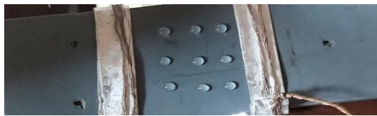
Figure 4: Photograph of the specimen with 9 droplets of water and electrodes for field application.
