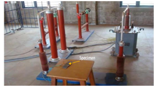
Figure 6: Experimental setup for measuring surface characteristics
