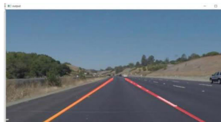
FIGURE 3: The left and Right lanes are detected.
