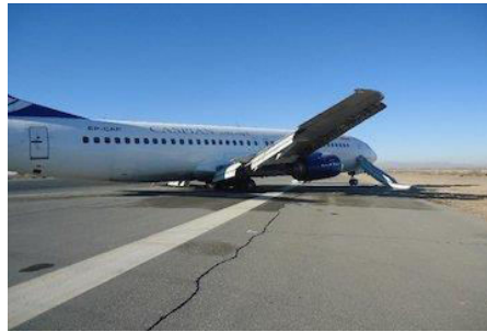
Figure 4. Landing with a technical fault of the landing gear
