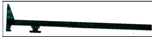
Figure 11. Finite element analysis model of coke pushing ram.
