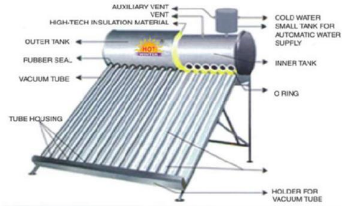
Figure 1- Components of the Solar Heater
