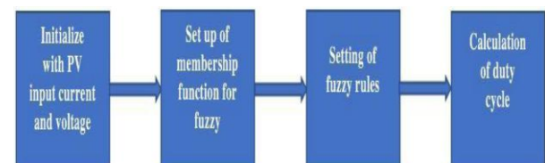
Figure 7. The fuzzy logic control is depicted as a block diagram.
