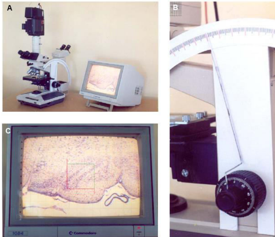
Figure 4. (A) The microscope set-up used to perform optical counting designs. It consists of a microscope (Olympus BH-2) and a color monitor (Commodore 1084). Beside the microscope is a part of a prepared circular scale and a pointer. (B) This part is fitted to the side of the microscope so that it shares the same center with the microscope's fine focus knob. The whole scale has a radius of 20 cm and contains 720 gradation marks. Each mark represents a vertical stage movement of 0.28 \mu\text{m} . The part of the scale used here has 210 gradation marks and represents a vertical traveling distance of about 60 \mu\text{m} . The angular displacement on the scale during the stage movement is read by a pointer which is fixed to the fine focus knob and moves together forward and backwards (C) The transparent indexed sheet superimposed on the monitor is used for field sampling and counting (see text and Figure 3 for its usage). It comprises steps for sampling fields (to be used at low magnification) and an unbiased counting frame (to be used at the evaluation magnification).
