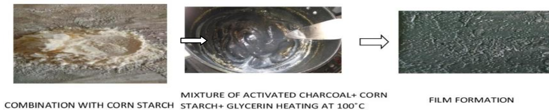
Figure.2. Shows a) the combination of corn starch, and b) combination of activated charcoal, corn starch and glycerin, c) formed film.
