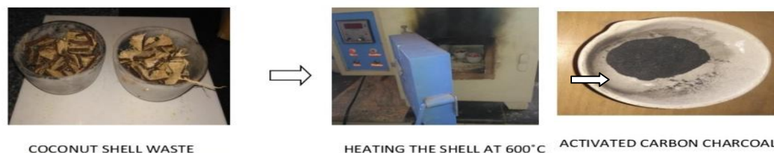
Figure.1. collected coconut shell waste heating at 600 °C and activated charcoal was produced
