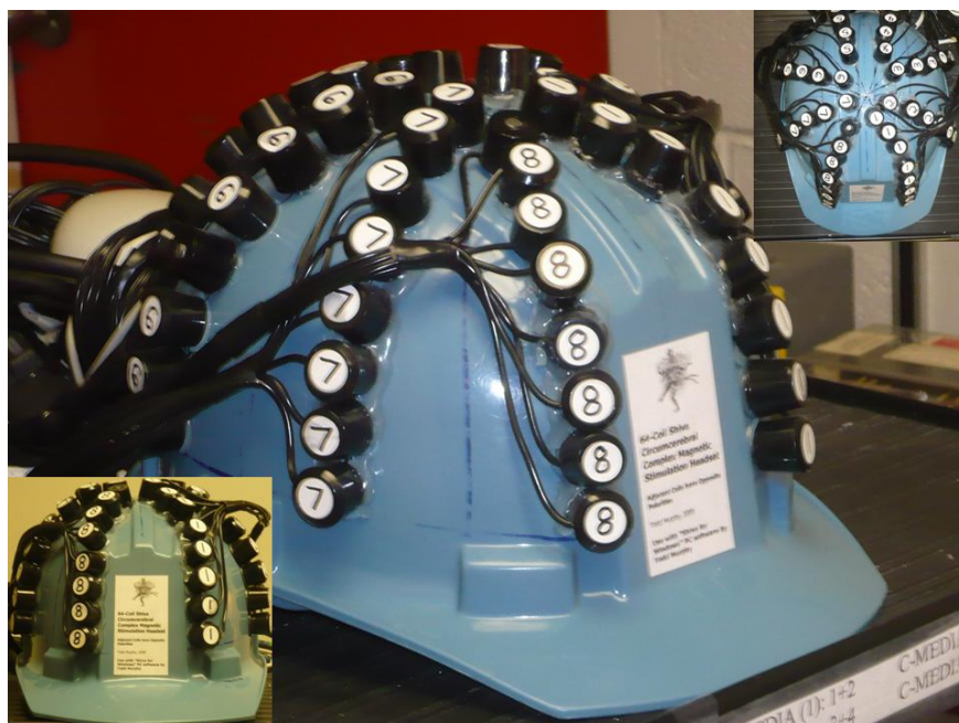
Figure 1. Lateral, frontal and topographical views of the custom-constructed hat used in the experiment. The hat contains 64 solenoids arranged in columns of 8 separated by 45 degrees.
