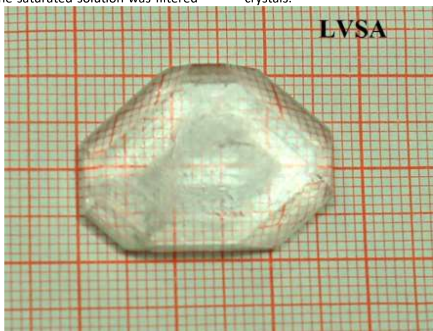
Figure 1. Photographs of the grown LVSA crystal
