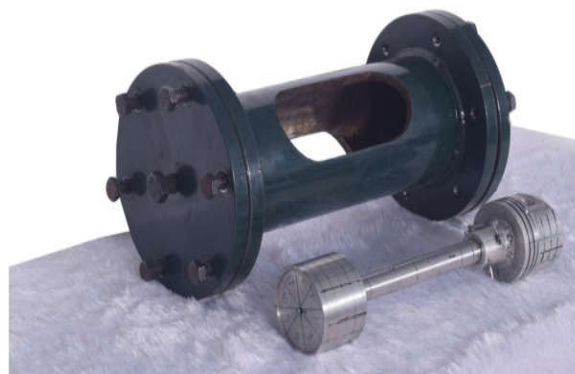
Fig. 1. Piston assembly with corresponding welding fixture.
