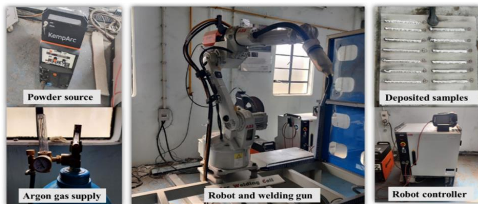
Fig. 2 Experimental setup of a robotic-controlled GMAW based-WAAM
