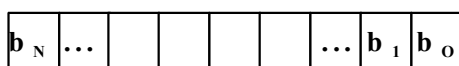
Figure 2. Specialized qubits comprising a word of savant processing memory ( b_0 is a flag qubit).
