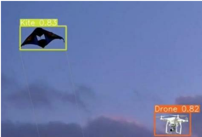
Fig. 8(d). Drone and kite detected
