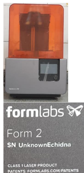
Fig.1. Form2 SLA 3D printers
