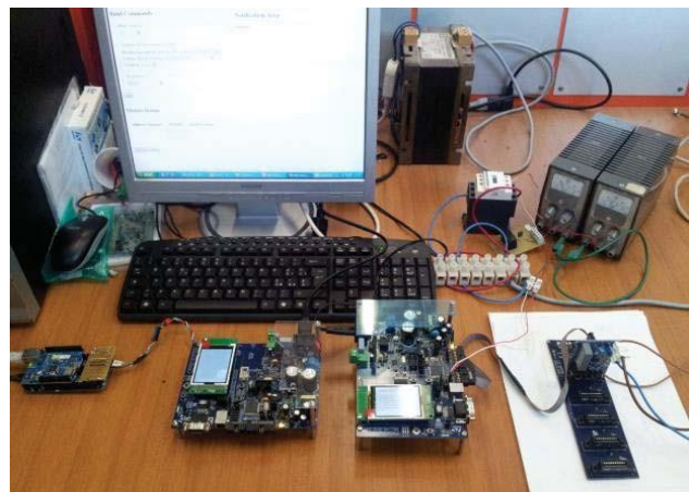
Fig. 3. Measurement set-up for IPR testing.
